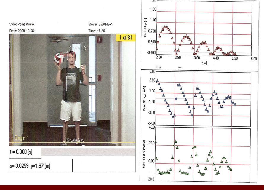
Movie analysis allows study of semi-elastic collision (types of collision, coefficient of restitution)
